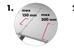
Space fixings not less than 10 mm from the panel edge – at 150 mm intervals round the edge and at 300 mm intervals elsewhere.
