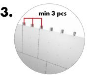
Each individual panel should always be supported by no less than three noggins.
