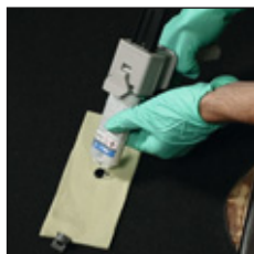
8. Remove the cap, ensure the pistons are working evenly and attach the nozzle.
