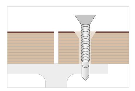
Countersinking according to screw head shape is recommended
